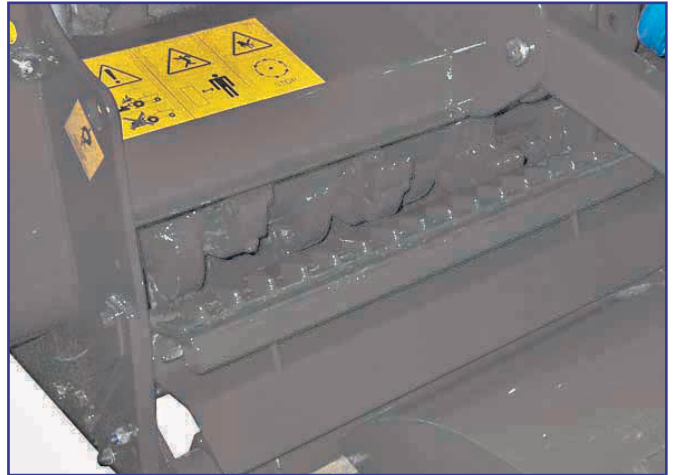
Two doors to access rotor and processing screen
