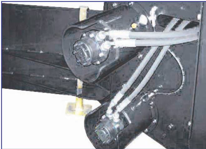
Two hydraulic motors power the feed rotors with protective casing
